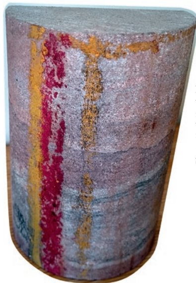
This core shows a good example of tramlines, with the red and yellow lines clearly marked on the outside. The red line should always be on the right.
