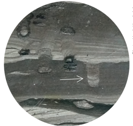
Close-up of a Ness core showing burrows that clearly indicate what the orientation of the core needs to be.
